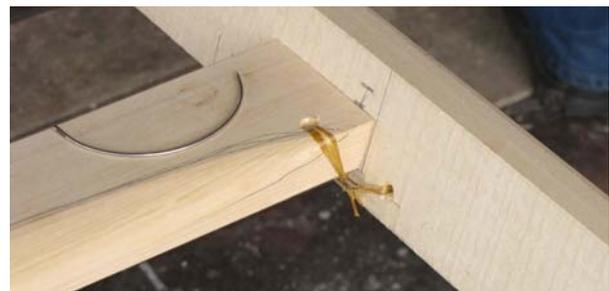
**Figure 13.** Lashing made easy using a curved needle
