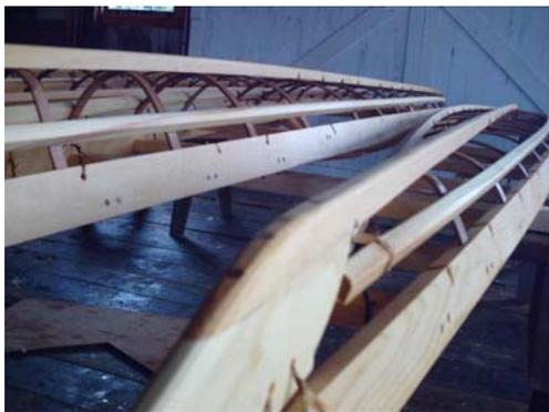
**Figure 18.** *Waiting for the waterproofing to dry (Note that the horizontal wood is the keel, chine and gunwale as you look down the upside-down kayak)*
