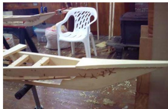
*Figure 7. Stabilising the frame to work on a stem piece*
