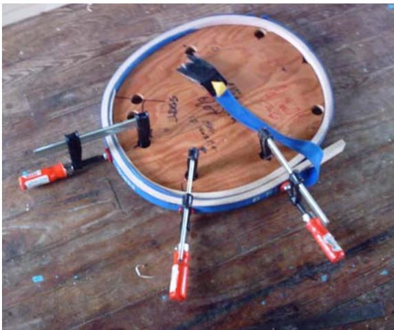
*Figure 10. Bending wood around a cockpit template to form a coaming*
